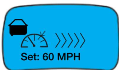
Cruise control set. ACC and CWS activated. No lead vehicle detected.
