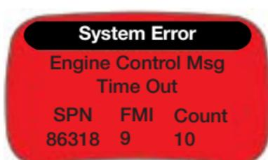
If there is a fault in the system, OnGuard will not emit collision warnings or apply Active Braking. If there is an active fault, the display will turn red and the fault code will appear. If this occurs, take the vehicle in for service as soon as possible (**fault information should be recorded for troubleshooting**). Your vehicle's cruise control system, including ACC, CWC and CMS, will not warn or function until the active fault in the system is corrected.
