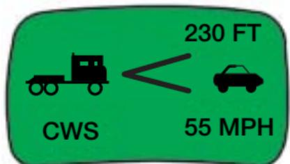
Cruise control not set. Lead vehicle detected.
