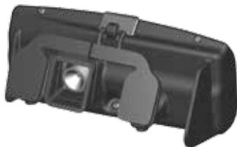
This Driver Tips Guide applies to vehicles equipped with the OnLane™ Lane Departure Warning System with SafeTraK technology by Takata. OnLane is a camera-based warning system that helps your driver avoid unintentional lane drifting.
