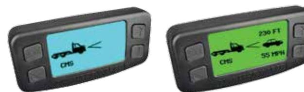
No lead vehicle detected. Lead Vehicle detected.
