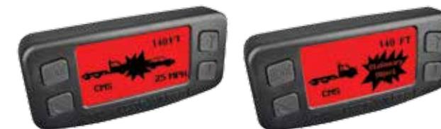
Object Collision Warning Stationary Object Warning
